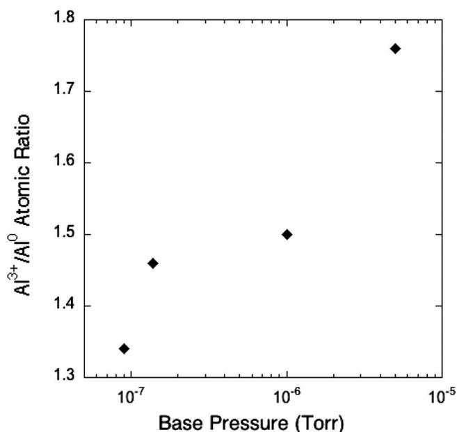
Figure 8. Al<sup>3+</sup>/Al<sup>0</sup> atomic ratio measured by XPS as a function of base pressure.
