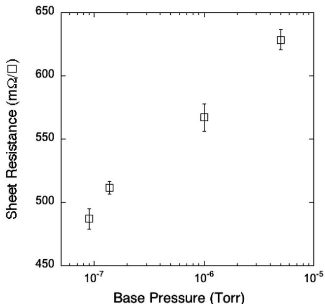
**Figure 5.** Forward sheet resistance measured for thin films as a function of base pressure.
