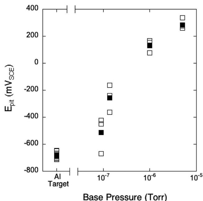
**Figure 2.** Summary of pitting potential data. Filled symbols represent average values and open symbols are data from all experiments performed on different samples.
