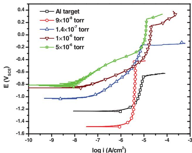
**Figure 1.** Potentiodynamic polarization anodic curves of Al target used for film sputtering, and Al films produced at different pressures in 0.1 M NaCl.
