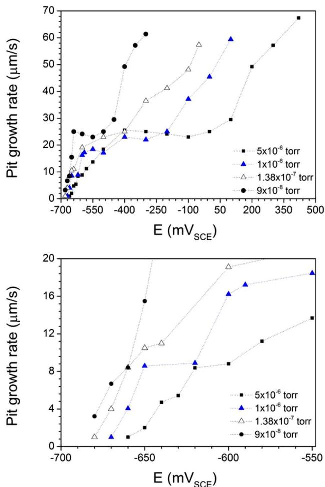
**Figure 6.** Thin film pit polarization curves in 0.1 M NaCl determined by image analysis of growing pits for thin films deposited with different base pressures. (a) full range of potential (b) region near repassivation expanded for clarity.
