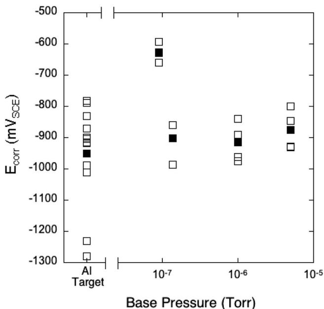
**Figure 3.** Summary of corrosion potential data. Filled symbols represent average values and open symbols are data from all experiments performed on different samples.
