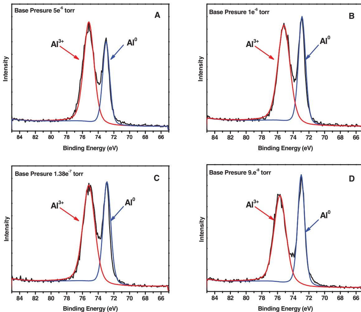
Figure 7. XPS high-resolution spectra of Al 2p for a)  $5 \times 10^{-6}$  torr, b)  $1 \times 10^{-6}$  torr, c)  $1.38 \times 10^{-7}$  torr and d)  $9 \times 10^{-8}$  torr.
