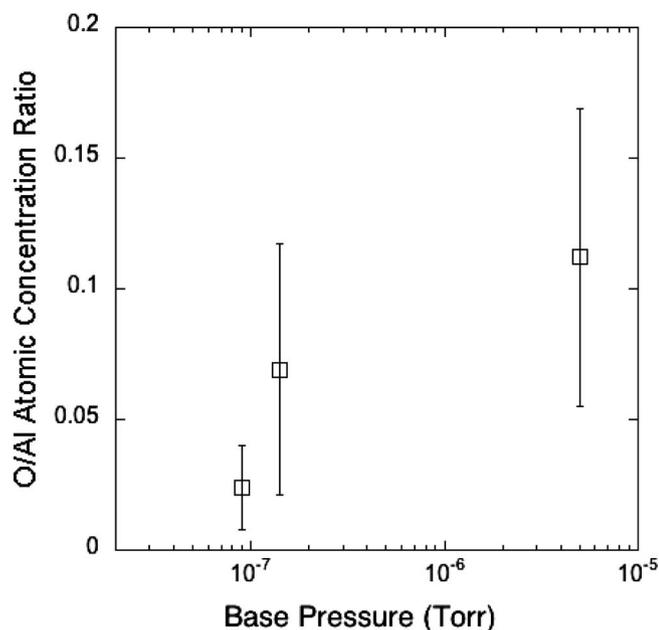
Figure 9. O/Al atomic ratio measured by DXDS as a function of base pressure.
