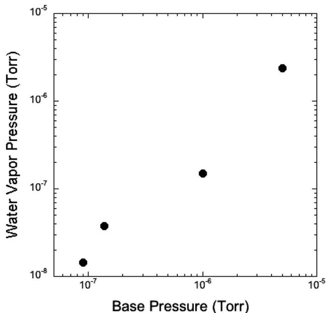
**Figure 4.** Water vapor pressure measured by residual gas analysis of the base vacuum as a function of base vacuum pressure.
