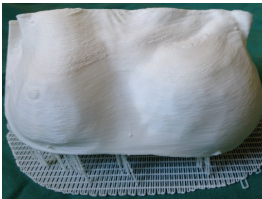
Figure 4: A three dimensional (3D)-printed haptic, tactile biomodel of the breast (same patient as Figure 1), produced from computed tomography (CT) data. Printing performed with the Cube 2 printer (3D Systems, Rock Hill, SC, USA) using Cubify software (3D Systems), and using white polylactic acid (PLA) filament ink. Reproduced with permission from: Chae MP, Hunter-Smith DJ, Spychal RT, Rozen WM. 3D Volumetric Analysis for Planning Breast Reconstructive Surgery. Breast Cancer Res Treat. 2014 June; [Epub ahead of Print].
