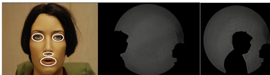
**Figure 2. Singapore experimental set-up, showing:** Swabbing sites for the manikin's face (A) for influenza testing. Shadowgraph images of far- (B) and near- cough (C) distances (see accompanying online Video S1 for further details of these shadowgraph images). doi:10.1371/journal.pone.0107338.g002
