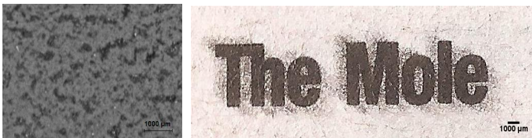
Fig. 1. Lint accumulation on the blanket is shown on the left hand side, and the right image shows the deterioration in the quality of the printed image as a result of lint accumulation.
