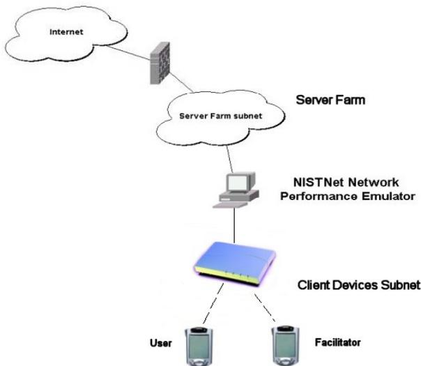
Figure 3: Wireless Data Network Test-bed used in Measuring Application-specific QoS in a Mobile Context
