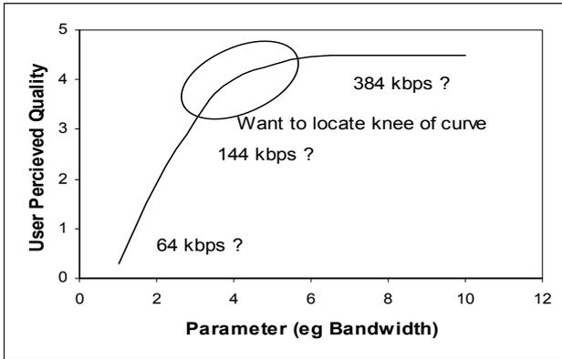
Figure 1 : An Example of a Quantitative Mapping Between Network Parameters and User-Perceived Quality of Service
