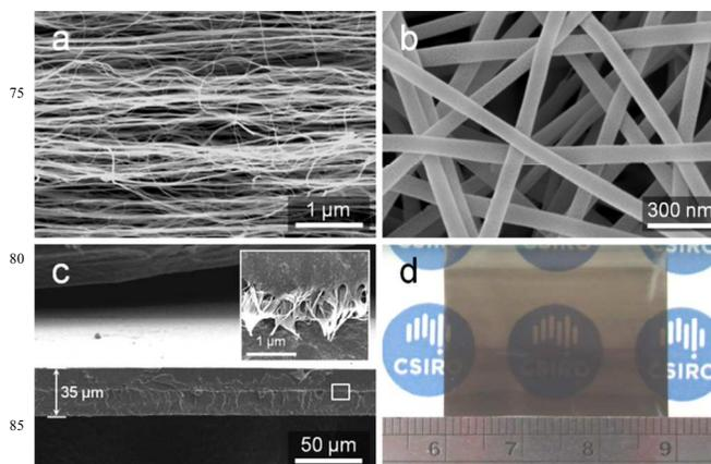
**Fig. 1** SEM images of the (a) dsCNT web, (b) electrospun SPEEK (c) cross-section of SPEEK/dsCNT membrane, with inset image showing higher magnification and optical image (d) of the SPEEK/dsCNT membrane.
