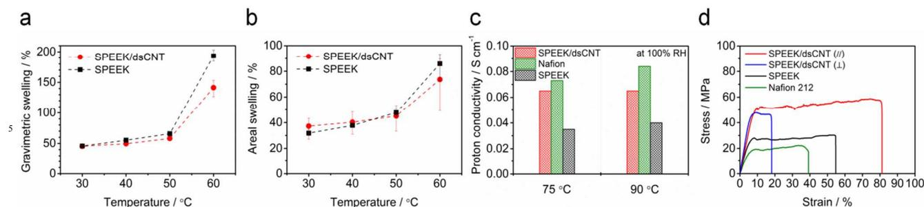
**Fig. 2** (a) Gravimetric and (b) areal swelling of SPEEK/dsCNT and SPEEK, and the (c) proton conductivity and (d) stress-strain of SPEEK/dsCNT (parallel and perpendicular to the dsCNT web layer), SPEEK and Nafion membranes.
