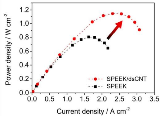
Text: A composite proton exchange membrane prepared by electrospinning SPEEK and direct spinning of CNTs is more robust than SPEEK alone and outperforms SPEEK and Nafion 212 membranes.
