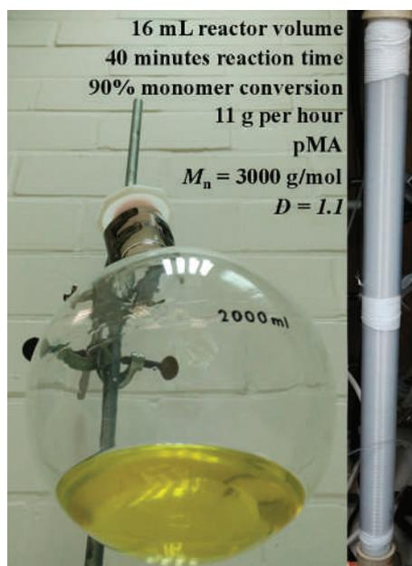
**Figure 4.** Photo of the tubular flow reactor with an internal volume of 16 mL (right) and the 200 g pMA obtained by collection of product over 18 h in the same reactor (left)
