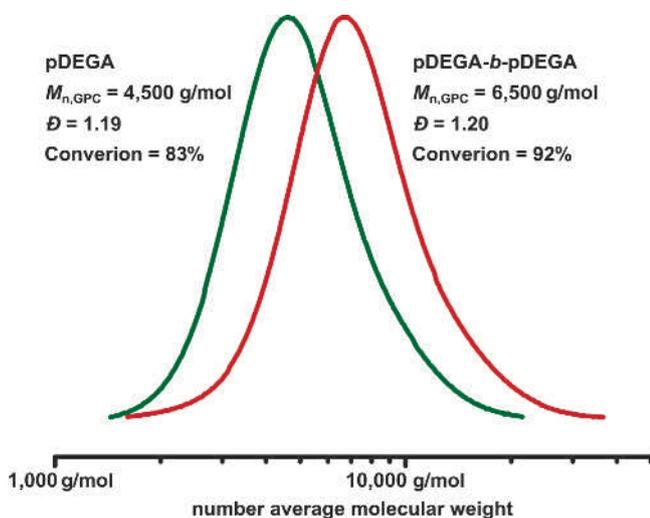
**Figure 6.** Molecular weight distributions of polymer obtained after the first and after the second reactor stage (both residence times set to 10 min per reactor coil)
