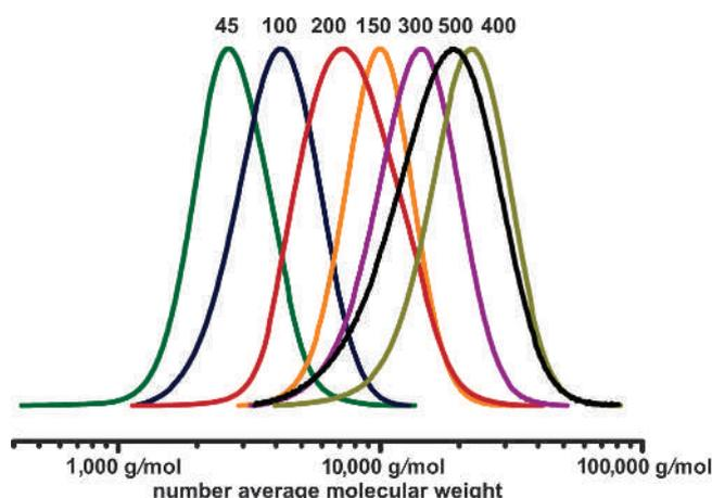
**Figure 2.** Molecular weight distributions for polymers made in continuous-flow photoCMP of methyl acrylate under variation of the initiator concentration in order to produce materials with different target molecular weight
