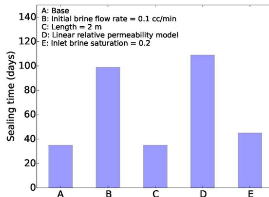
Fig. 7. Predicted sealing times for a 100 μm fracture when the reactive surface area is proportional to the brine saturation. The base case corresponds to an initial brine flow rate of 0.05 cc/min, length of 1 m, Corey relative permeability model, and an inlet brine saturation of 0.5. For the remainder four simulations all variables, except for the variable noted in the legend, were set equal to the values for the base case.
