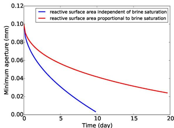
Fig. 6. Comparison between the sealing time of a 100 μm fracture when the reactive surface area is independent of the brine saturation and when the reactive surface area is proportional to the brine saturation. (For interpretation of the references to color in this figure, the reader is referred to the web version of this article).
