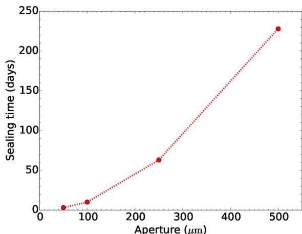
Fig. 5. Sealing time for fractures with different apertures. In all four simulations the reactive surface area is assumed to be independent of the brine saturation.
