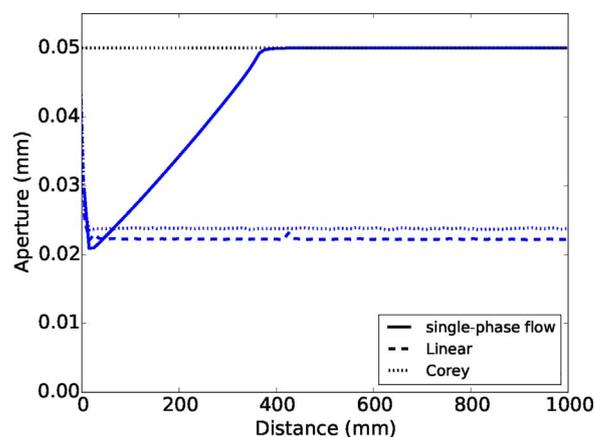
Fig. 2. Model predictions of the location of the calcite precipitate layer in the fracture for single-phase and two-phase simulations (using the linear and Corey relative permeability model). The dashed black line indicates the initial location of the fracture surface. (For interpretation of the references to color in this figure, the reader is referred to the web version of this article).
