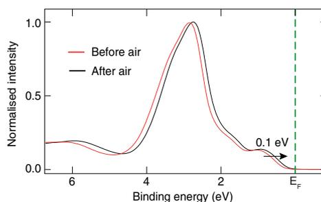
**Figure 4.** Valence band spectra of N implanted  $\text{Cu}_2\text{O}$  before and after being exposure to atmosphere, collected using synchrotron radiation ( $h\nu = 100 \text{ eV}$ ).
