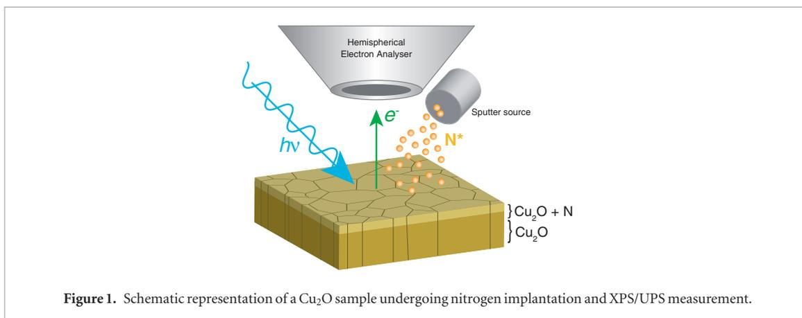
**Figure 1.** Schematic representation of a Cu<sub>2</sub>O sample undergoing nitrogen implantation and XPS/UPS measurement.
