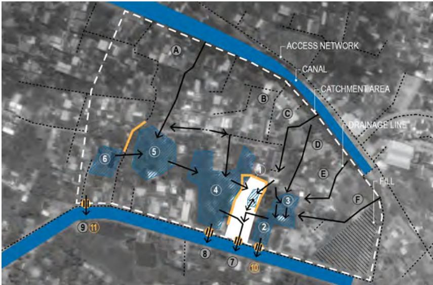
**Figure 7:** Flood protection strategies at Precinct and site levels. The Precinct is marked with a dashed white line, and the pilot site is shaded in white. Waterways and catchments are indicated in solid and hatched blue, respectively, and improvements such as floodwalls and culverts in yellow.
