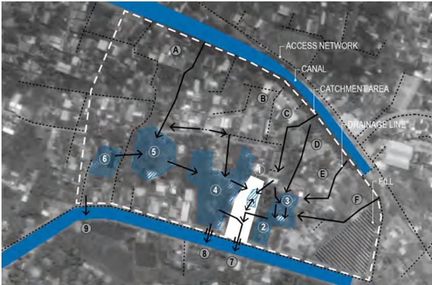
**Figure 2:** The Precinct is marked with a dashed white line, and the pilot site is shaded in white. Waterways and catchments are indicated in solid and hatched blue, respectively, and existing culverts discharging to stormwater canal (not all functional) are shown at 7, 8, and 9.
