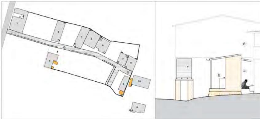
**Figure 9:** [Left] Wetpod strategy illustrated in plan shows new wetpods in orange, provided to buildings 3, 9 and 10. [Right] Section showing a wetpod with detached rainwater tank adjacent to an existing building.
