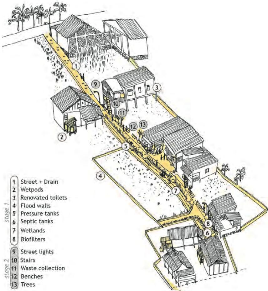
**Figure 5:** Axonometric of the water-sensitive cities approach for Batua, Makassar. Intervention in yellow, illustrating Stage 1 elements funded by ADB and Stage 2 elements funded by local government.
