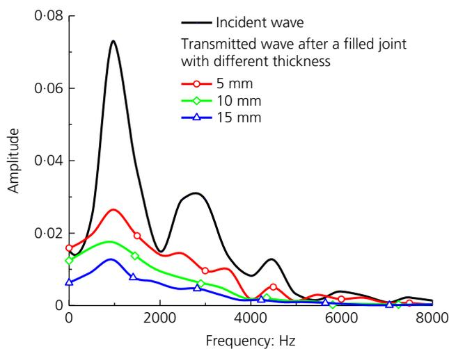
Fig. 6. Frequency spectrum of the incident wave and transmitted waves after different thickness joints
