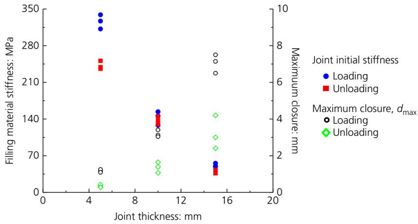
Fig. 4. Joint stiffness and maximum closure under loading/unloading processes at different joint thicknesses
