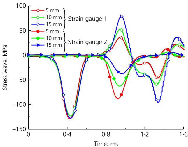
**Fig. 2.** Stress waves on the incident and transmitted bars at identical gas pressure for 5, 10 and 15 mm thickness filled joints
