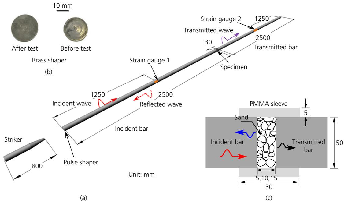
**Fig. 1.** (a) Schematic diagram of the SHPB apparatus for high-amplitude seismic wave propagation across a sand-filled joint, (b) brass pulse shaper and (c) sleeve configuration
