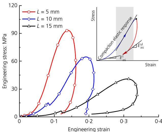
**Fig. 3.** Stress–strain response of dry sand fillings at 5, 10 and 15 mm thickness under dynamic loading
