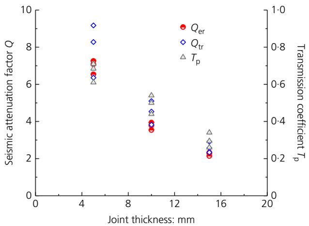
Fig. 5. Wave transmission coefficients as a function of joint thickness
