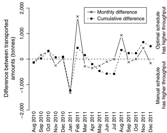
**Figure 4:** The graph compares tonnage transported using the optimal and manual schedules. The continuous line shows the difference between the monthly transported amounts for these schedules. The dashed line shows the difference in cumulative tonnage. The cumulative difference at the end of the planning period is positive, which means that the optimizer outperforms the manual schedule.
