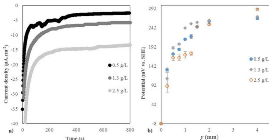
**Fig. 6** **a** Cathodic potentiostatic responses for varying initial cupric ion concentrations, potential set to  $-8$  mV versus SHE, pore length set to  $l = 10$  mm. **b** Potential profile along the  $l = 10$  mm diffusion pore at varying initial cupric ion concentration. Measurements were taken immediately after the termination of the polarization phase
