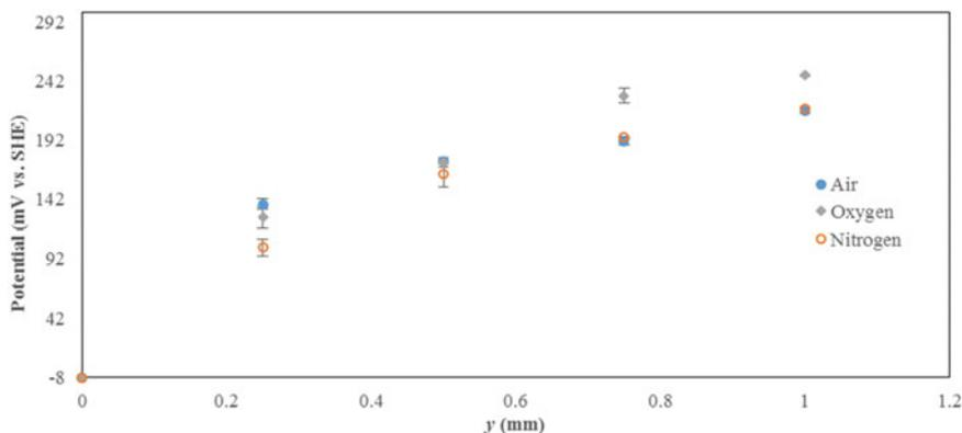
**Fig. 7** Potential profile along  $l = 10$  mm diffusion pore in varying concentrations of oxygen
