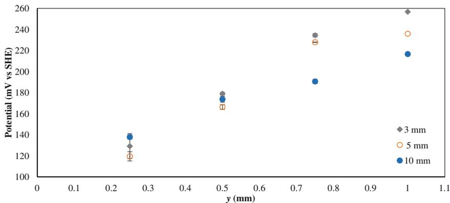
**Fig. 5** Potential profiles generated along varying diffusion pore lengths ( $3 < l < 10$  mm,  $0.25 < y < 1$  mm). Measurements taken after immediate conclusion of the cathodic polarization phase
