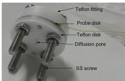
Fig. 2 Experimental model cell for an encapsulated ore particle
