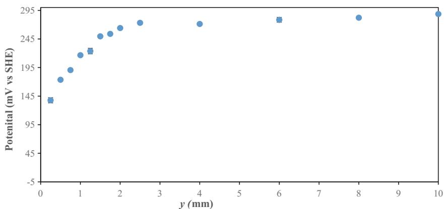
**Fig. 4** Potential profile along the fixed length ( $l = 10$  mm) diffusion pore. Potential measurements were taken after immediate termination of the cathodic surface polarisation
