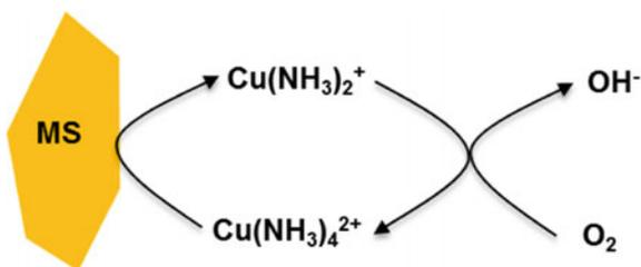
surface. The hindered mass transport of these species results in concentration gradients within the pore. The potential of the system is related to the activities (estimated as concentrations in dilute solutions) of the oxidised and reduced species present in that solution, through the Nernst equation. In the presence of ammonia, the equilibrium potential was computed by Meng and Han [7] to incorporate complexation with ammonia:
