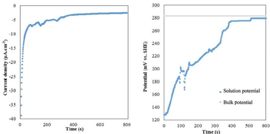
**Fig. 3** **a** Cathodic potentiostatic test, potential set at  $-8$  mV versus SHE in a solution with base operating conditions,  $l = 10$  mm, (Pt-E reaction surface area =  $0.02356$  cm<sup>2</sup>). **b** Solution potential measured by a platinum probe placed at  $y = 0.25$  mm from the reaction surface in an  $l = 10$  mm diffusion pore, under base operating conditions. Measurement began immediately after terminating the cathodic reaction at the surface
