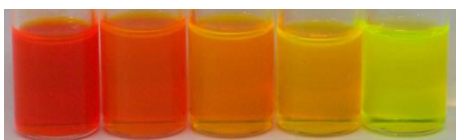
Figure 1. Photograph showing the colours of dichloromethane solutions as a function of TIPS-DBC concentration (from left to right: 10, 5, 2.5, 1.25, 0.125 mM).
