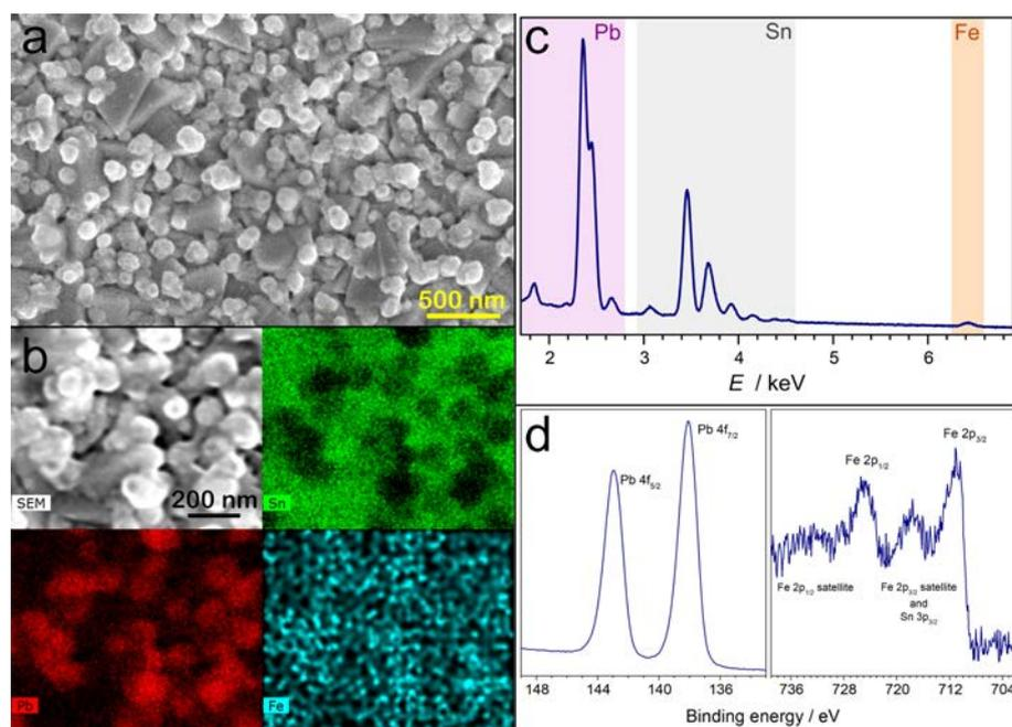
**Figure 4.** Characterisation of the electrodeposit produced during oxidation of aqueous  $225 \mu\text{M Fe}^{2+} + 10 \mu\text{M Pb}^{2+}$  (with  $0.2 \text{ M Na}_2\text{SO}_4$ , pH 2.9) at  $2.03 \text{ V vs. RHE}$  for 20 min with a FTO electrode: (a) SEM image, (b) EDX mapping, (c) EDX spectrum, (d) Pb 4f and Fe 2p spectra.
