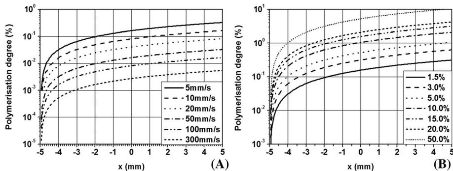
**FIGURE 2** Effect of (A) laser speed and (B) laser power on polymerisation degree of 5.0 wt% GnP/epoxy nanocomposite. The laser power was set to 1.5% for results in (A) and the laser speed was 5 mm/s for (B)
