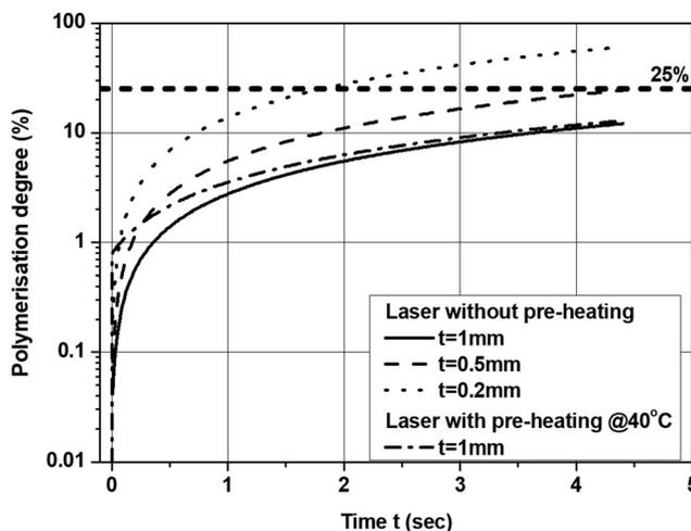
**FIGURE 4** Polymerisation degree on scanning area of 1 mm × 1 mm with different thicknesses and including material preheating effect in function of time
