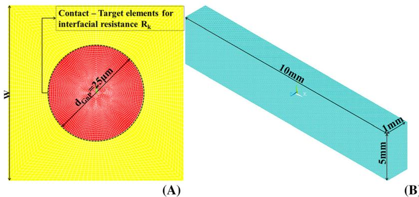
**FIGURE 1** A, Unit cell top view with unit cell width  $w$  and GnP particle diameter  $d_{\text{GnP}} = 25$  μm. B, Cuboid specimen model of nanocomposite with surface of 10 mm  $\times$  5 mm and thickness of 1 mm
