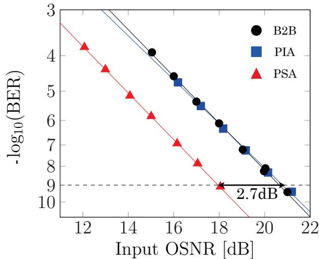
Fig. 5. BER curves at high noise loading.
