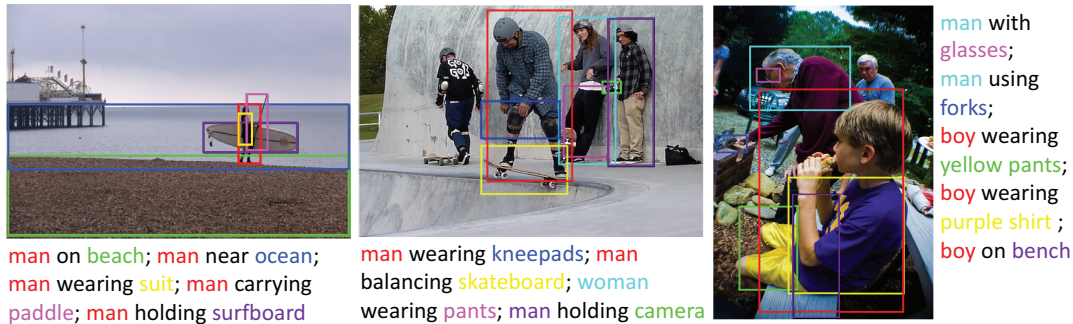
Figure 4: Qualitative examples of the predicate detection. The color of human and objects in the phrases correspond to the color of the bounding boxes. We only predict the interactions between the ground-truth bounding box pairs.
