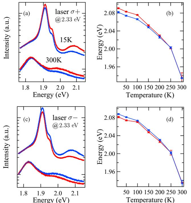
FIG. 3. PL spectra of the MoS<sub>2</sub> ML at different temperatures. (a),(c) Optical spectra at 15 and 300 K pumped by a right- and left-handed circularly polarized laser, respectively. The experimental data is shown by circles, the fitting curves are shown using lines. Power density: 0.048 MW/cm<sup>2</sup>. (b),(d) Exciton energy against temperature.
