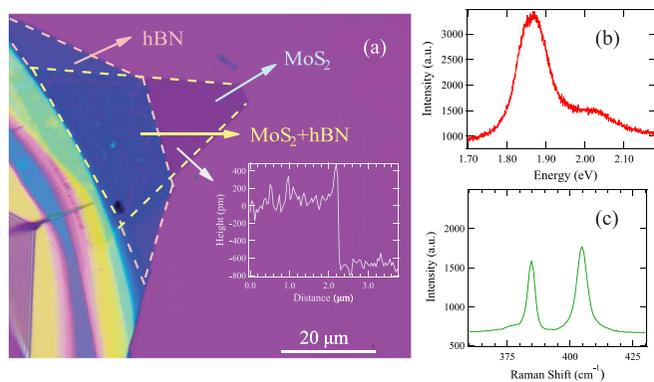
FIG. 1. Optical characterization of the sample. (a) The optical image and the AFM mapping of the MoS<sub>2</sub> ML, where the inset shows the thickness of the sample is about 0.7 nm. (b) PL spectrum of the MoS<sub>2</sub> ML excited by a 532-nm laser at room temperature. (c) Raman spectrum of the sample at room temperature.
