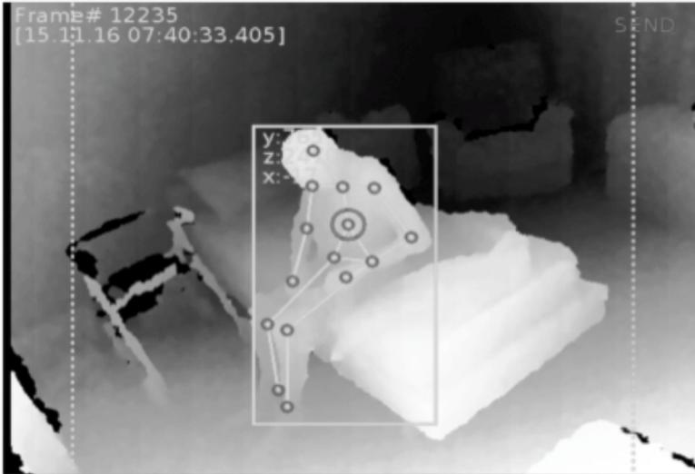
**Figure 1.** Example of a depth image map generated by the smart sensor system (Image courtesy of Sematrix Pty Ltd).
