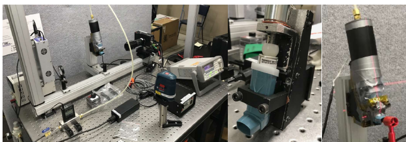
Figure 2 – (left) Spray analysis experimental apparatus: LED on the left, inhaler in the centre, camera on the right; (middle) pMDI plus Clip-Tone and solenoid plunger; (right) turbine rotameter in front of the pMDI mouthpiece.
