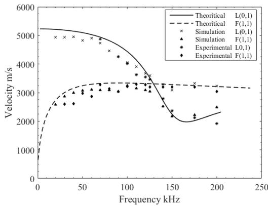
Figure 1 Dispersion curves for a rod that is 20 mm in diameter, showing longitudinal and flexural modes.
