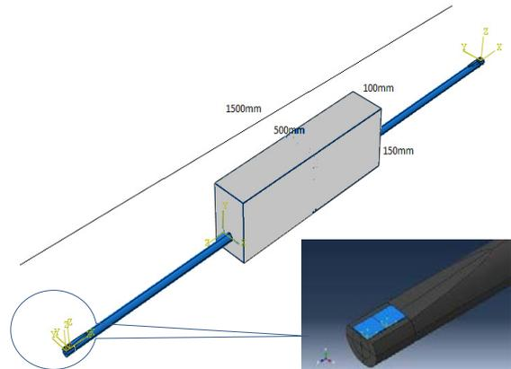
Figure 2 Schematic diagram of the reinforced concrete beam that was used in study of corrosion and de-bonding.
