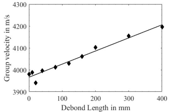
Figure 9 Variation of velocity of L(0, 1) mode with increase in debond between steel and concrete
