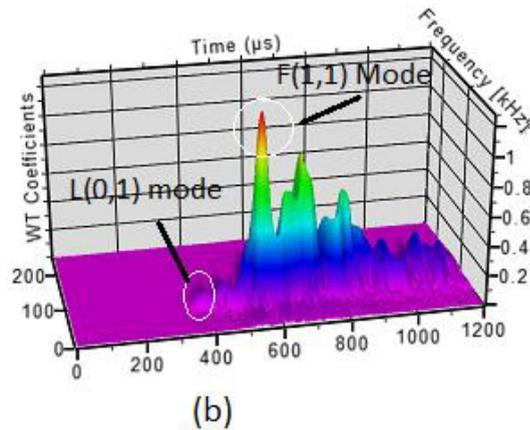
Figure 3 Response of an undamaged structure at 100 kHz excitation frequency (a) Time History (b) 3D plot of signal using Gabor wavelet
