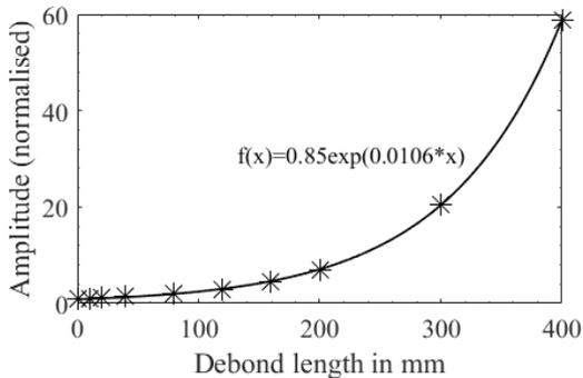
Figure 8 Variation of amplitude of L(0, 1) mode with increase in debond between steel and concrete
