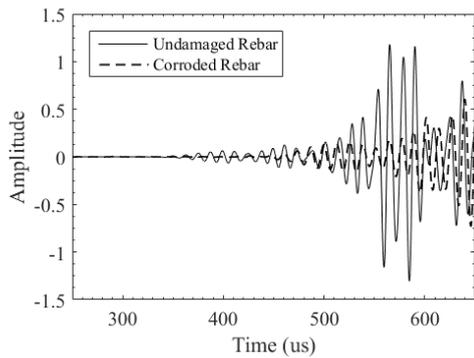
Figure 4 Comparison of signals received in an undamaged specimen and a corroded specimen
