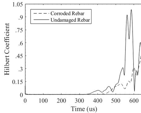
Figure 5 Energy envelope of an undamaged specimen and a specimen subjected to corrosion
