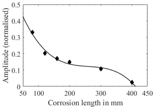
Figure 6 Variation of amplitude of L(0, 1) mode with corrosion along the length of the rebar.
