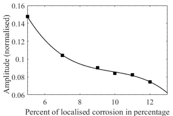
Figure 7 Variation of amplitude of F(1, 1) mode with pitting type of corrosion in the rebar.
