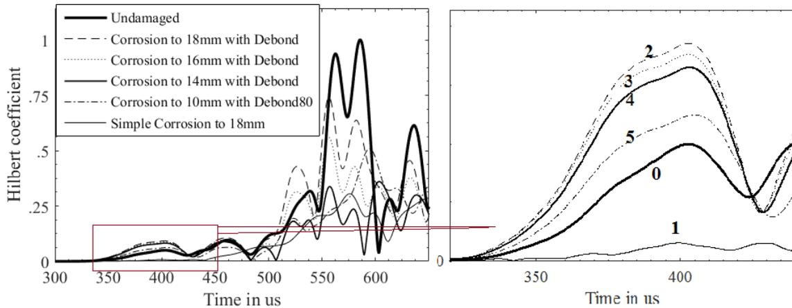
Figure 10 Comparison of energy envelopes for various damage scenarios, in order to identify the zero state effect for damage that is located at the centre of the rebar.
