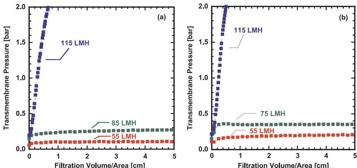
Fig. 5. The effect of permeate flux on fouling of PS20 UF membranes modified with: (a) PMPC 2 g/L and PD 2 g/L for 0.5 h (PD-PMPC-1) and (b) 2 g/L of PMPC and 5 g/L of PD for 0.5 h (PD-PMPC-4). Constant flux fouling experiments at 55, 75, 85 and 115 LMH were performed with a 1500 ppm soybean oil emulsion feed (3 samples per experimental set). The data presented is from the cell with intermediate TMP values. Feed pressure: 2.1 barg, crossflow velocity: 0.18 m/s (Re = 1000).
