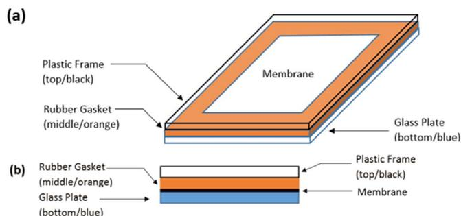
Fig. 1. (a) The front view and (b) the cross-sectional view of the membrane modification module employed in these studies.
