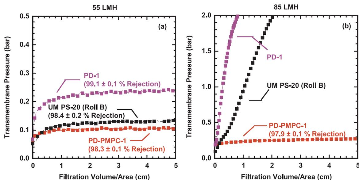
Fig. 6. Constant flux comparison of unmodified PS20 Roll B, PS20 modified with PD 2 g/L 2.5 h (PD-1), and PS20 modified with PMPC 2 g/L PD 2 g/L 0.5 h (PD-PMPC-1) at: (a) 55 LMH and (b) 85 LMH. Constant flux fouling experiments were run with a 1500 ppm soybean oil emulsion feed. Each experiment tested 3 samples, and the plot presented is of the cell with intermediate TMP values. Feed pressure: 2.1 barg, crossflow velocity: 0.18 m/s ( $Re = 1000$ ).
