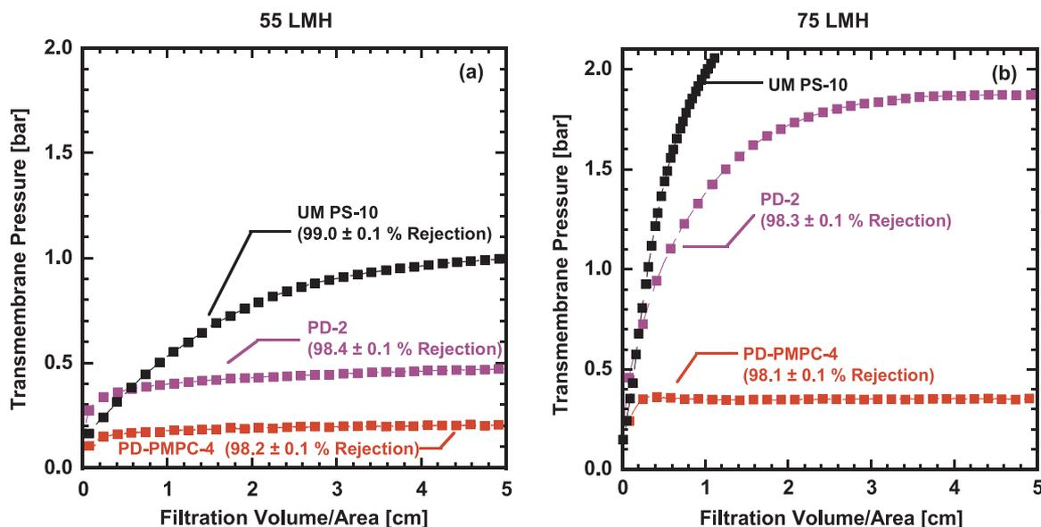
Fig. 7. Constant flux comparison of unmodified PS10, PS20 modified with PD 4 g/L 1.5 h (PD-2), and PS20 modified with PMPC 2 g/L PD 5 g/L 0.5 h (PD-PMPC-4) at: (a) 55 LMH and (b) 75 LMH. Constant flux fouling experiments were run with a 1500 ppm soybean oil emulsion feed. Each experiment tested 3 samples, and the plot presented is of the cell with the intermediate TMP values. Feed pressure: 2.1 barg, crossflow velocity: 0.18 m/s ( $Re = 1000$ ).
