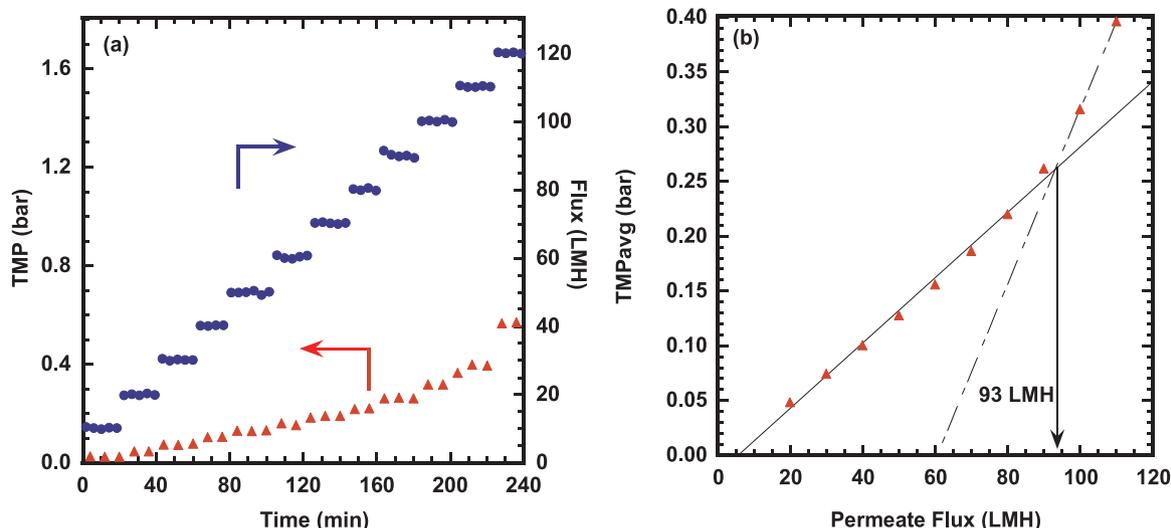
Fig. 4. Threshold flux determination of modified UF membranes (PD-PMPC-1) challenged with 1500 ppm soybean oil emulsion field. (a) Flux stepping experiment with stepwise flux increase by 10 LMH every 20 min. Initial Flux: 10 LMH. Feed pressure: 2.1 barg, crossflow velocity: 0.18 m/s (Reynolds number (Re) = 1000); (b) Threshold flux determination. The average TMP of each flux step is plotted against permeate flux. The threshold flux value is shown by the arrow pointing to the permeate flux axis.
