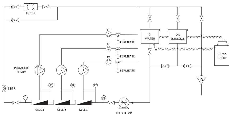
Fig. 2. Schematic of the crossflow fouling system employed in this work. (PT- pressure transducer, FT- flow transducer, BPR- back pressure regulator, D- drain).
