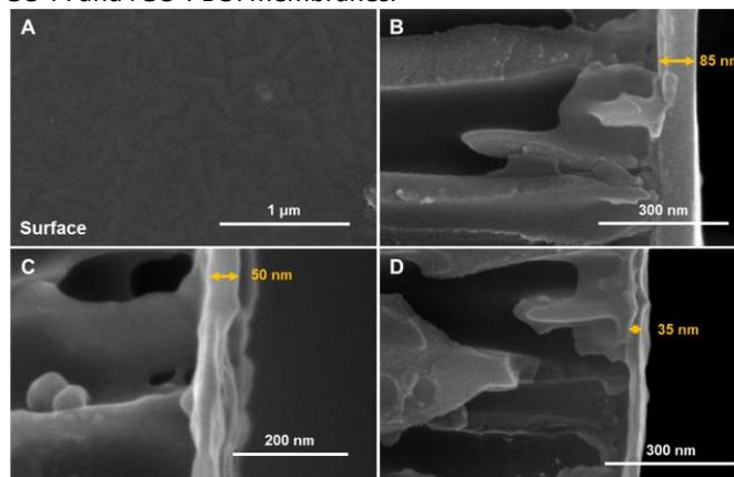
**Fig. 2** SEM images of rGO-PBOI-2.0 membranes prepared from the solution in THF with a concentration of (a), (b) 5.0 wt%, (c) 2.0 wt%, and (d) 1.5 wt%.
