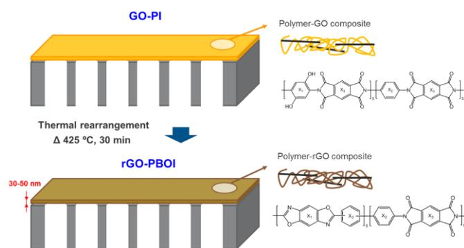
**Fig. 1** Schematic of the polymer-GO composite membranes.
