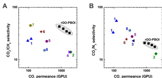
**Fig. 4** Gas permeance and selectivity of rGO-PBOI membranes from single gas experiments with a comparison to literature data (1: GO,<sup>28</sup> 2: TR-PBO,<sup>44</sup> 3: Crosslinked TR-PBOI,<sup>45</sup> 4: PBT-PEG,<sup>41</sup> 5: PIM,<sup>46</sup> 6: PIM-Matrimid<sup>®</sup>,<sup>46</sup> 7: Crosslinked PI,<sup>47</sup> 8: Pebax/IL<sup>48</sup>).
