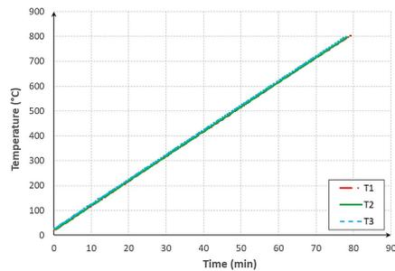
Figure 3. Thermocouple readings of a typical specimen
