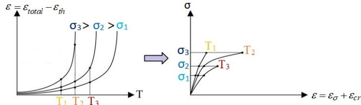
Figure 5. Procedure to find stress-strain curves including creep effects
