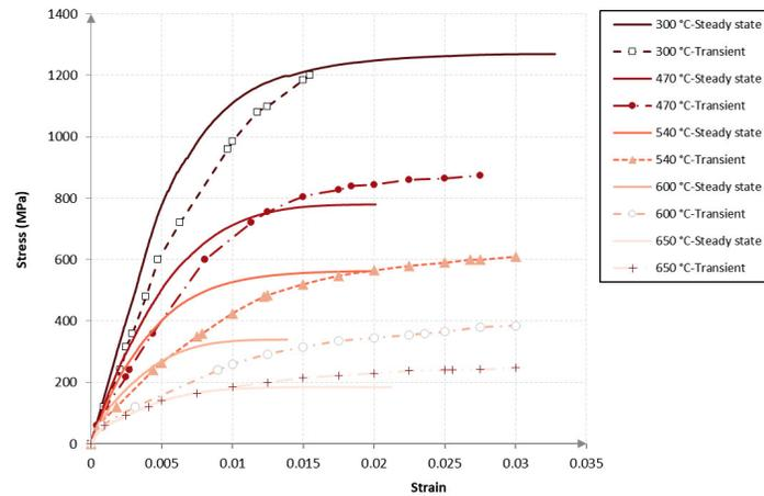
Figure 6. Stress-strain diagrams of Grade 1200 UHSS tubes at elevated temperatures using steady-state and transient testing methods
