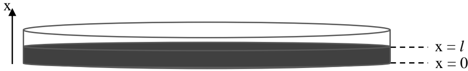
Figure 1. Schematic representation of diffusion occurring through a thin binder film in a circular dish.
