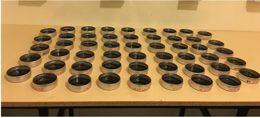
Figure 2. Evaporation test: metal dishes containing 2 mm thin bitumen/solvent binder films kept on table inside a controlled temperature room to continue testing for 1 month.
