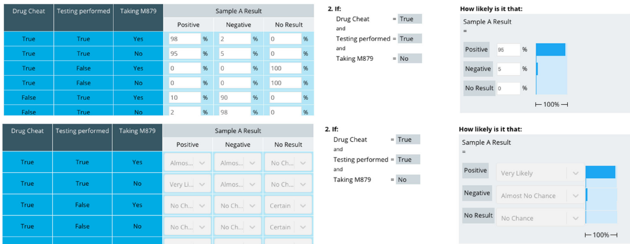
Fig 4. Examples of the four input modes available in Step 4 Parameters: percentages above, qualitative descriptors below; table left and question-based right.
