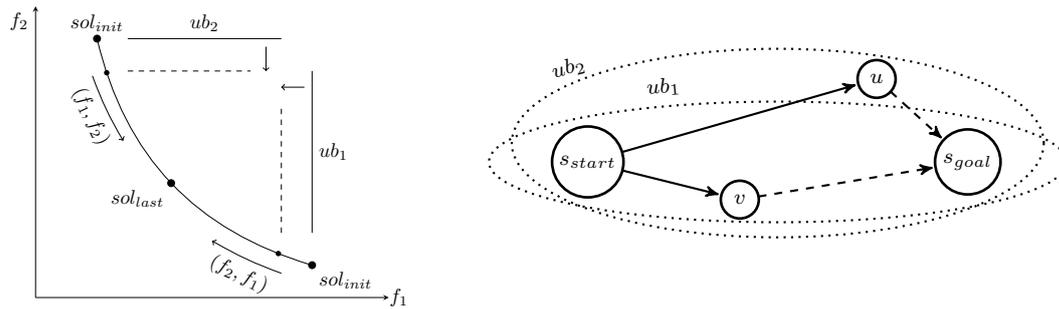
■ **Figure 1** Left: Objective orders, bounds and Pareto-optimal solutions. Right: Schematic of states outside or inside of upper bounds. State  $u$  is out of bounds for  $f_1$  and will be discarded in  $f_2$  search.
