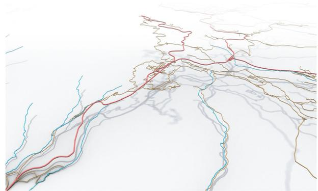
**Figure 3.** Roads and rivers rendered as 3D tubes over a flat white plane. Each class of line feature has a different color and radius. Terrain is absent but the shadows on the 'floor' give an indication of relative feature height.
