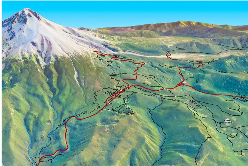
**Figure 4.** Final result for 3D roads and rivers. The flattened tube profile results in roads that are occluded by hills, but have a consistent and smooth appearance even in rugged terrain, with a slight perspective effect.
