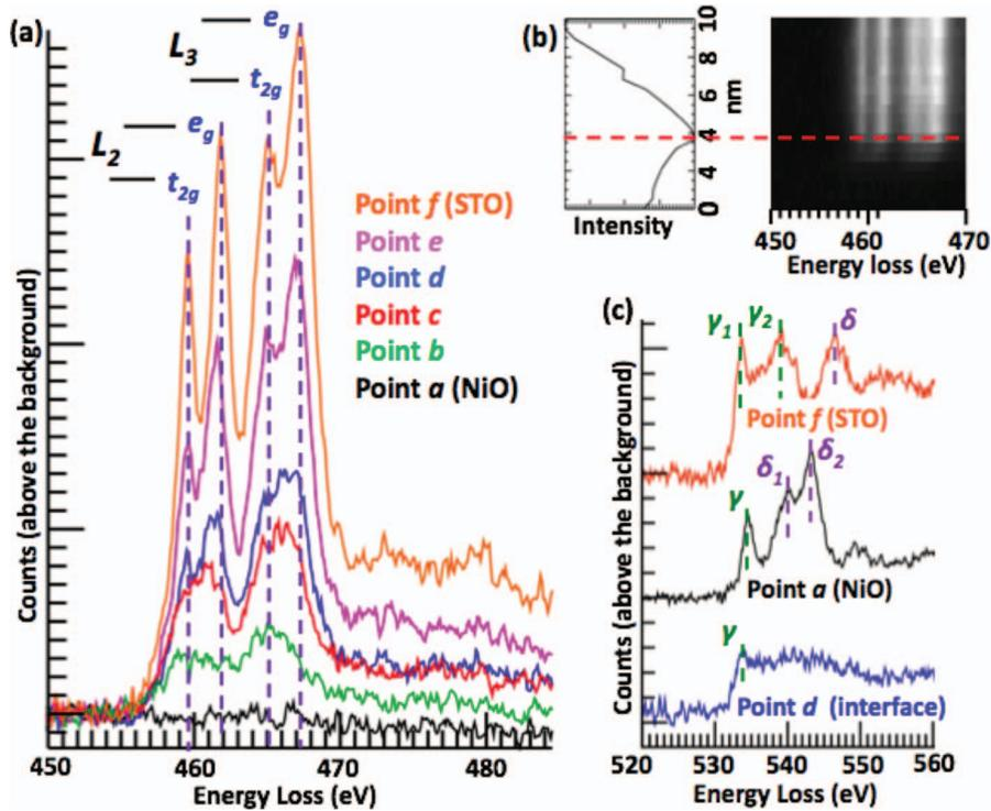
FIG. 3. (a) Ti  $L$  edges of the selected points (points  $a$  to point  $f$  as shown in Figure 2(b) and 2(d)) from EELS line scan. (b) ADF intensity plot and EEL spectrum image simultaneously acquired with EELS. (c) Simultaneously acquired O  $K$  edges from point  $a$ ,  $d$ , and  $f$ .
