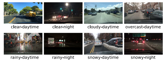
Fig. 5. Samples of BDD dataset, where source domain is clear-daytime, and target domains are clear-night, cloudy-daytime, overcast-daytime, rainy-daytime, rainy-night, snowy-daytime, and snowy-night.
