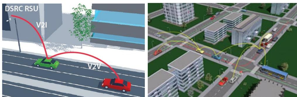
Figure 1: Examples of Vehicle-to-Vehicle and Vehicle-to-Infrastructure communications (figure from Cohda Wireless, 2009a and ITR, 2009)
